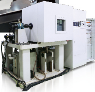
3Axial B/J Durability Tester
