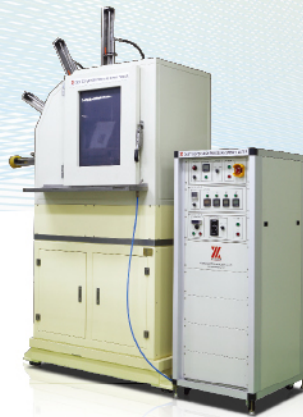
OBJ Dust Cover High Pressure Spray Tester
